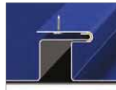
Typical 1 Reveal For 12" Panels
